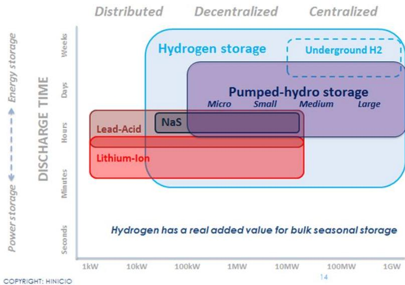
Hydrogen can provide storage solutions from 10 kW up to above 10MW, where batteries are no longer cost-effective
