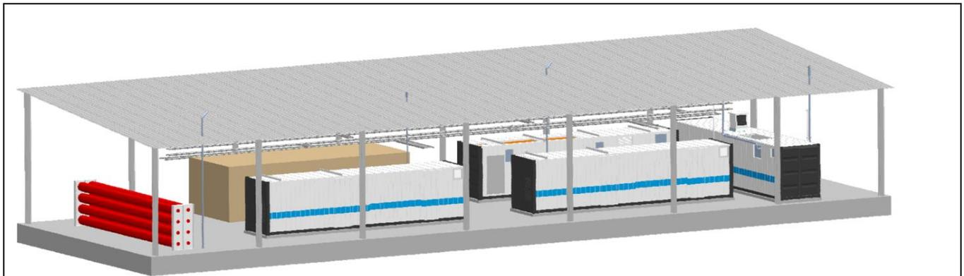
Hydrogen based energy storage system consisting of a 1 MW PEM electrolyzer, a 3 MWh hydrogen storage and a 300 kW fuel cell, stabilizing the power grid in Thailand (for EGAT) with high penetration of wind energy (source: Hydrogenics)
